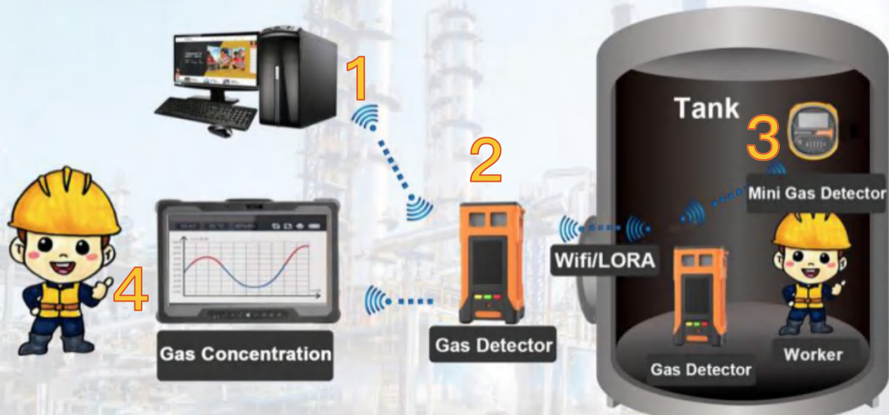
Schematic diagram of wireless transmission scheme in limited space (tank)
