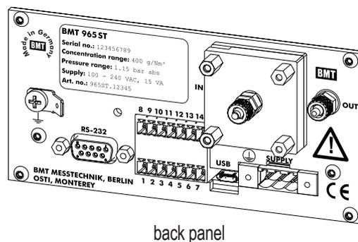
The OZONE ANALYZER BMT 965 is a panel-mount instrument according to DIN IEC 61554. The front panel cut-out should be 139 x 67 mm. The instrument is held in place by two clamps.
