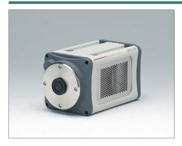
The ORCAII has a specialty feature of low noise and high-sensitivity. Cooling down enables dark current as low as 0.0012 electrons/pixel/second and the 1024  $\times 1024$  pixels BT-CCD (Back-thinned CCD) provides 1M pixel resolution and high quantum efficiency of over 90 % peak and broad sensitivity from UV to NIR.
