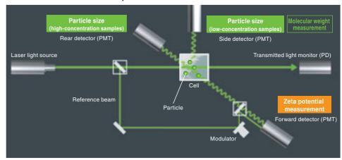
The optical configurations shown can be automatically selected depending on the concentration of the analyzed sample.
